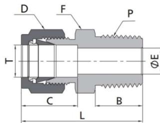
英制管-RT外螺纹/Fractional Tube to RT Thread
